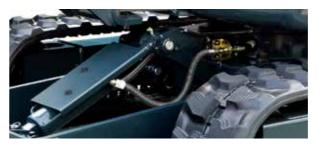
Two-Piece Hose for the Dozer Cylinder Two piece hoses were applied for a better and easier maintenance.
