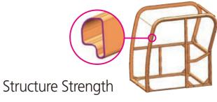
The 9A series cabin structure has been fitted with stronger but slimmer tubing for more safety and improved visibility. Low-stress, high strength steel is integrally welded to form a stronger, more durable upper and lower frame. Structural integrity was tested by way of FEM (Finite Elements Method) analysis and long-term durability tests.
