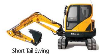
R60CR-9A's short tail swing radius allows the operator work in confined areas like close to buildings on roadways, and in urban areas. This compact radius design provides easy and efficient operation in any limited space work environment.
